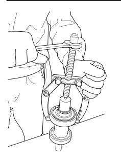
(6) Use a puller to remove ball bearing (321.1)(321.2) from drive shaft. Be careful not to scratch the sliding surface between drive shaft and shaft seal (420).
