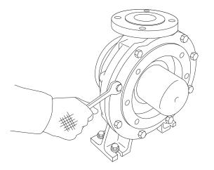
(8) Remove hex. bolts (901.4) of front casing (100.1) to pull out rear casing support.
