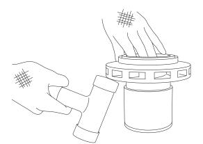
(4) Remove impeller (230) from magnet capsule (859). If it is hard to remove, slightly strike the impeller back side with plastic hammer.
