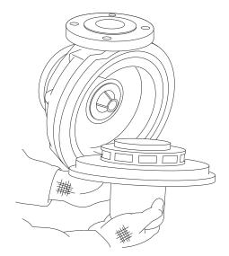
(9) Then, remove rear casing (158) from rear casing cover (159). If rear casing is hard to remove, remove it by turning. Pay attention not to drop the impeller (230)/magnet capsule (859) unit which is located in the rear casing.
